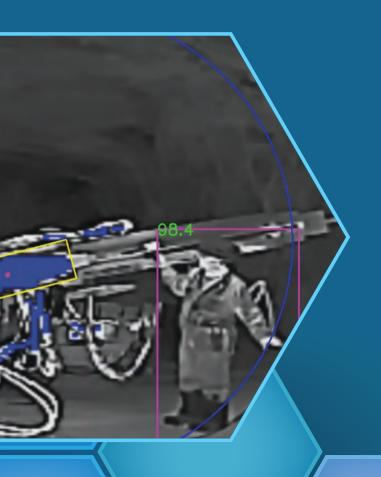
The system operates continuously, in real time, to detect people or machinery entering the danger zone. Unlike other systems that use lasers or other technology to detect people crossing a defined perimeter or "virtual fence", *Drill Sentry* provides continuous monitoring rather than detecting an intrusion event. This means the system cannot be defeated by resetting it after somebody has crossed the perimeter, therefore monitoring is ongoing.
